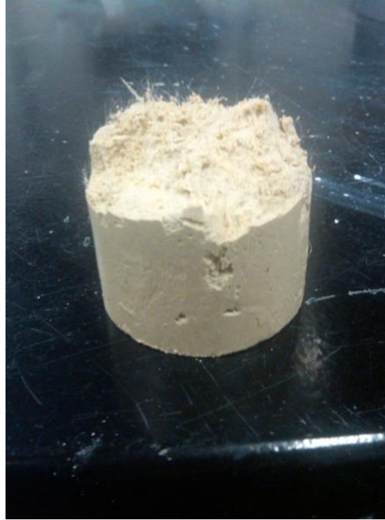
Figure 3.1. Example Distribution of Nylon Fibers through a Specimen
